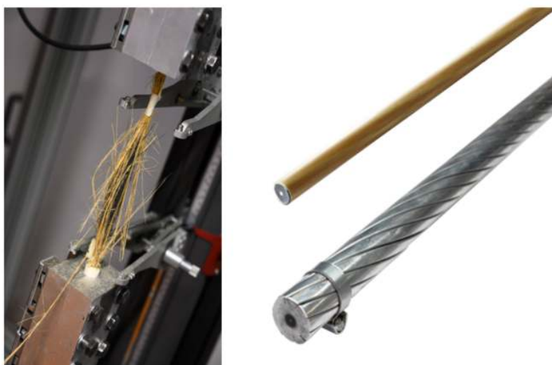
Figure 1 – composite core after tensile testing (result approx. 200 kN/45 kips), conductor (credit: Epsilon Cable)
