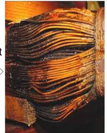
Transformer Winding Insulation Failure
