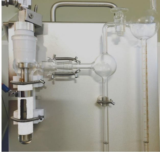
Figure 1: Example of the test cell and burette assembly used in IEC 60628 Method A – “Gassing Tendency”. This test is not related to stray gassing
