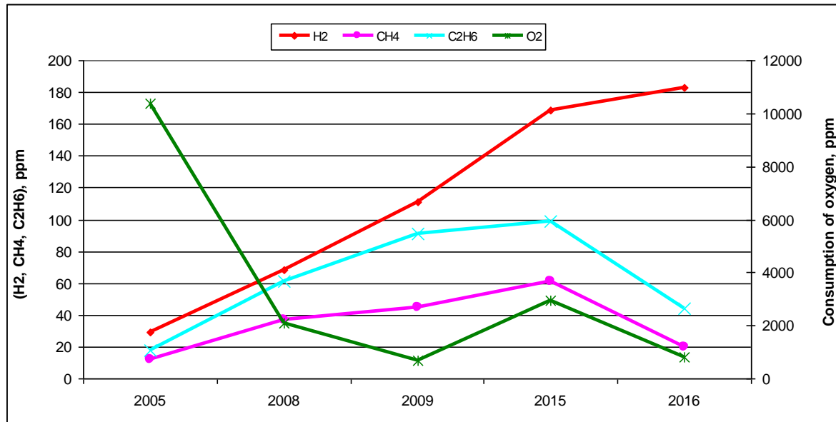
Figure 12 Development of the gas concentrations in the oil during the service
