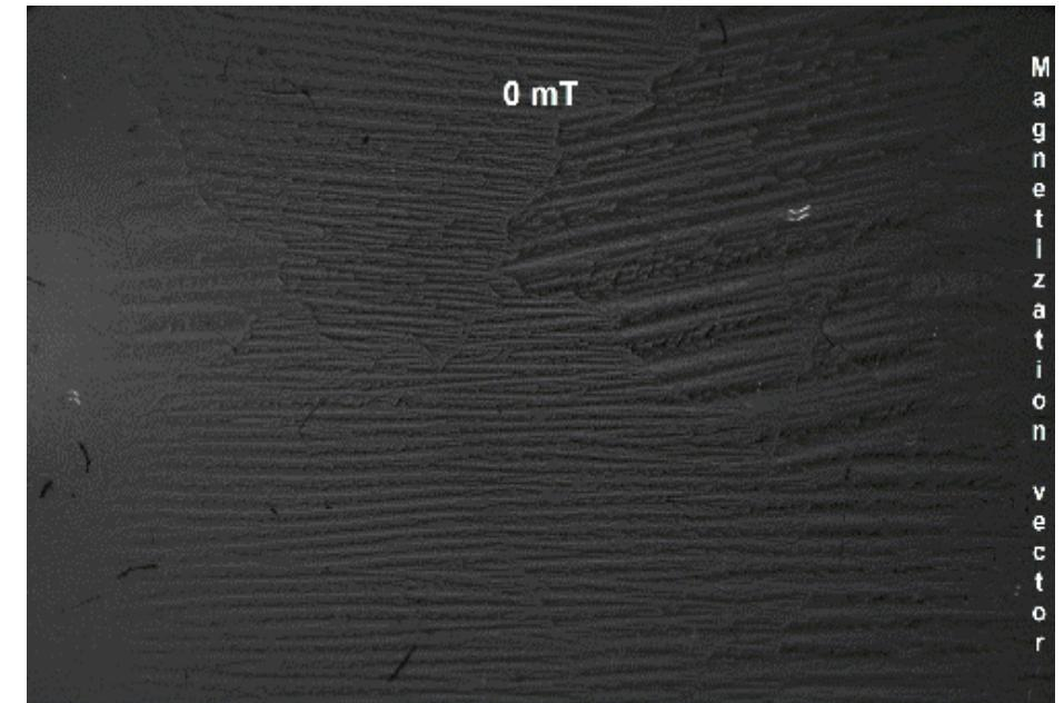
Grain oriented electrical steel sample placed inside an electromagnet. Magneto-optical images recorded with the CMOS-MagView; Source: Matesy GmbH
