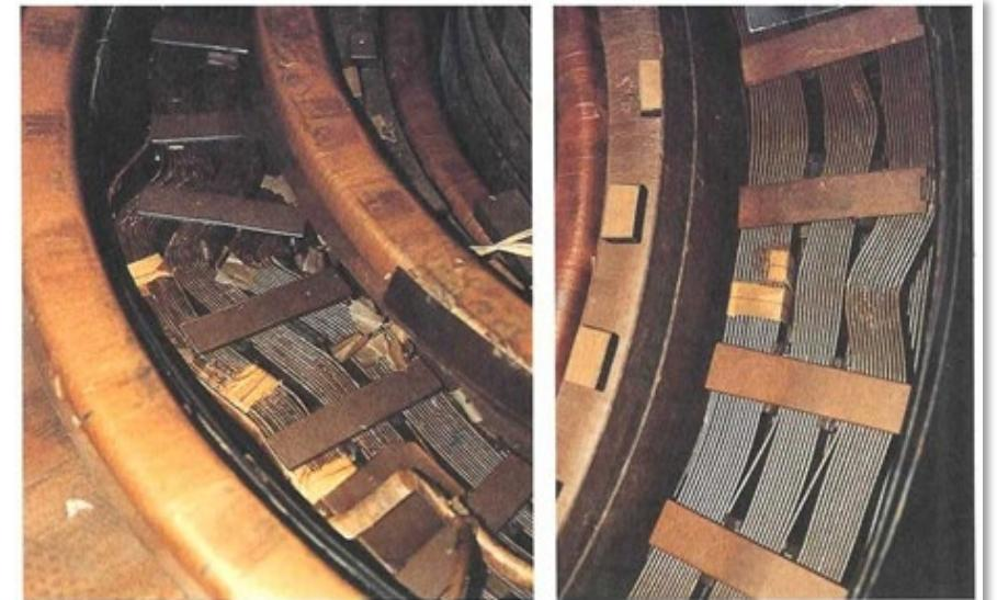
Winding deformation (buckling) causing a change of leakage flux
