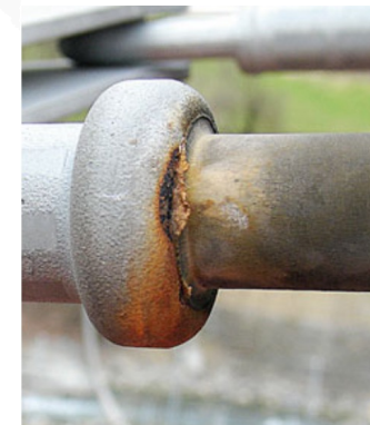
Damage caused by WDIC (Ref: Silicon Composite Insulators Book)
