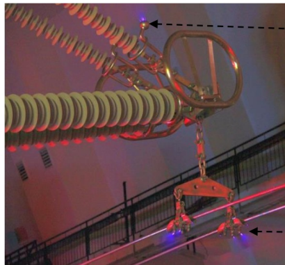
Test voltage: 300 kV (visible corona pattern predicted by FEA)
