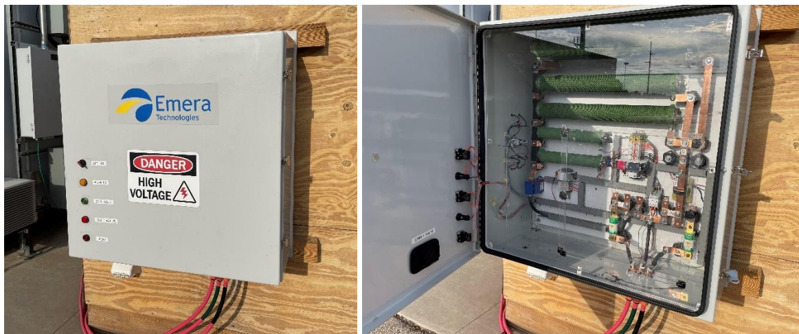
Fig. 6. Fault emulator hardware installed onto microgrid distribution bus at the DETL.
