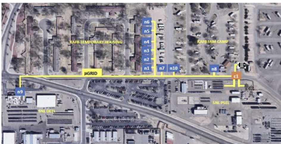
Fig. 1. KAFB DC microgrid serving housing, utility, and DETL sites.
