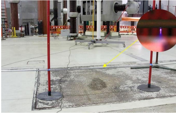
Figure 26. Test arrangement and corona inception on calibration sphere mounted on single conductor.
