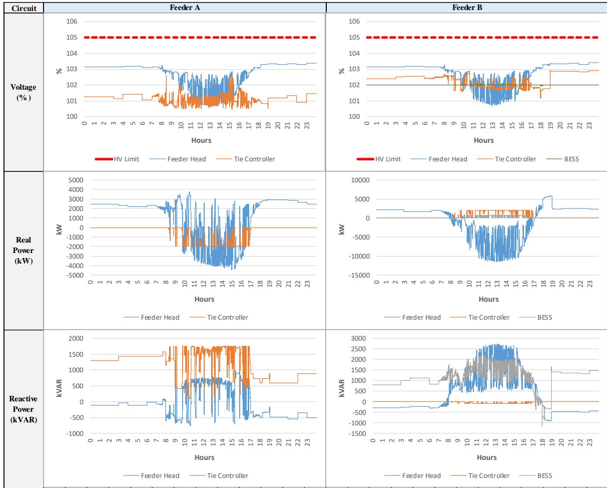
Figure 5: Time Series Plots for Tie Controller + BESS (Smart) Variant During Light Load Day
