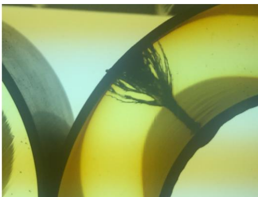
Figure 5: Hot-oil bath showing fault channel created by dielectric failure event. Specific root cause evidence most likely consumed by the withstand test fault.
