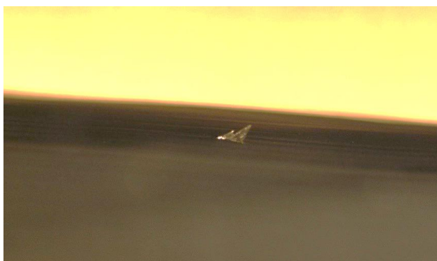
Figure 6: 10 \mu\text{m} void in XLPE insulation at the inner semicon screen of an installed cable found using a factory-comparable PD commissioning test with better than 5pC sensitivity. A withstand test would have destroyed this evidence.
