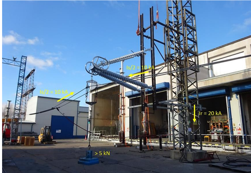
Figure 13. Arrangement for power arc test of insulated cross arm.
