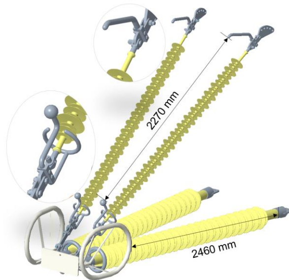
Figure 6. Power arc protection on the composite insulated cross arm.
