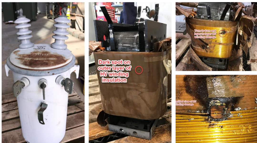
Figure 4. Images from forensic analysis of transformer failure. Starting from left going clockwise.
