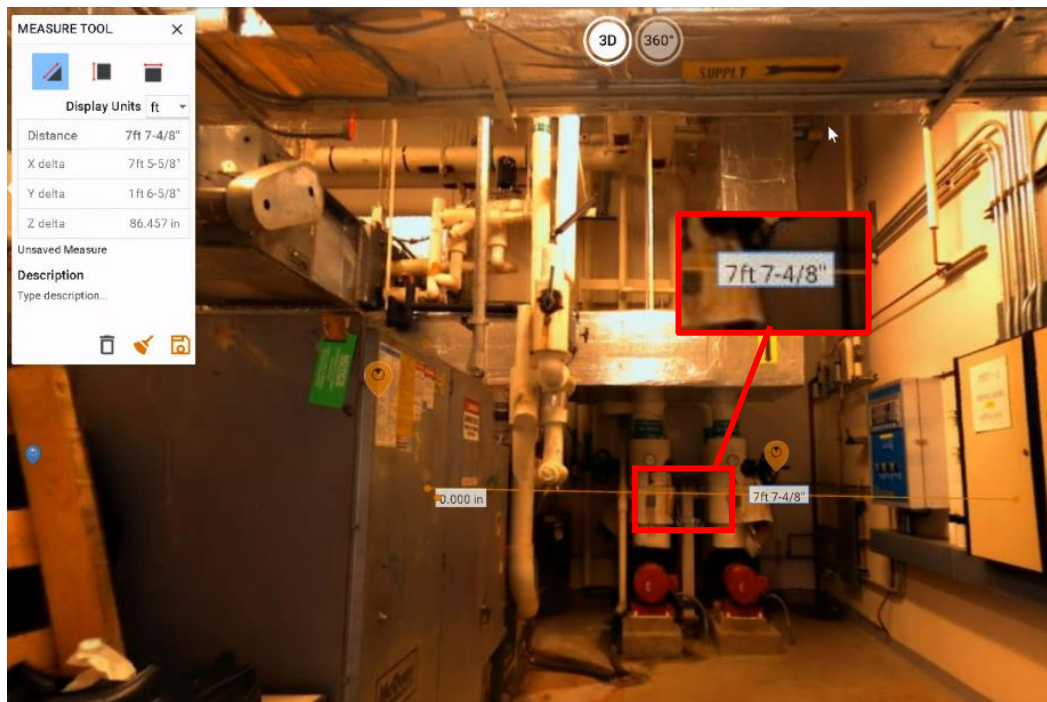
Figure 10: A screen capture of the Trimble 3D model software, illustrating the point-to-point dimensional measurement capabilities.
