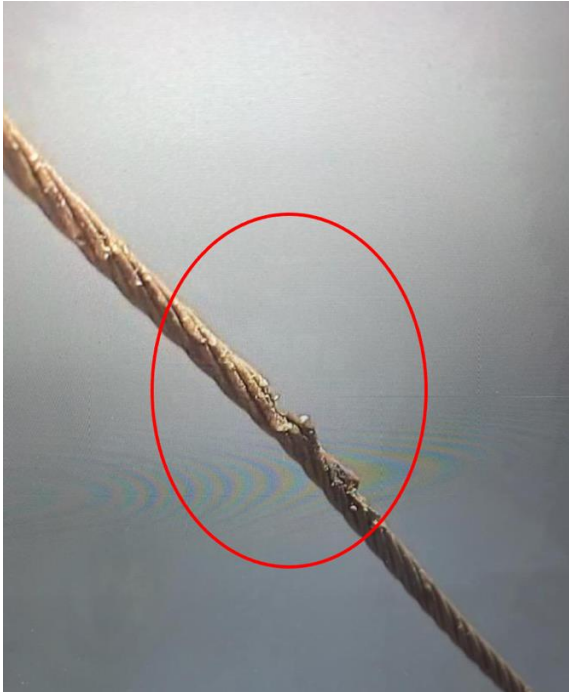
Figure 4 – Damage from Phase-Phase Contact
