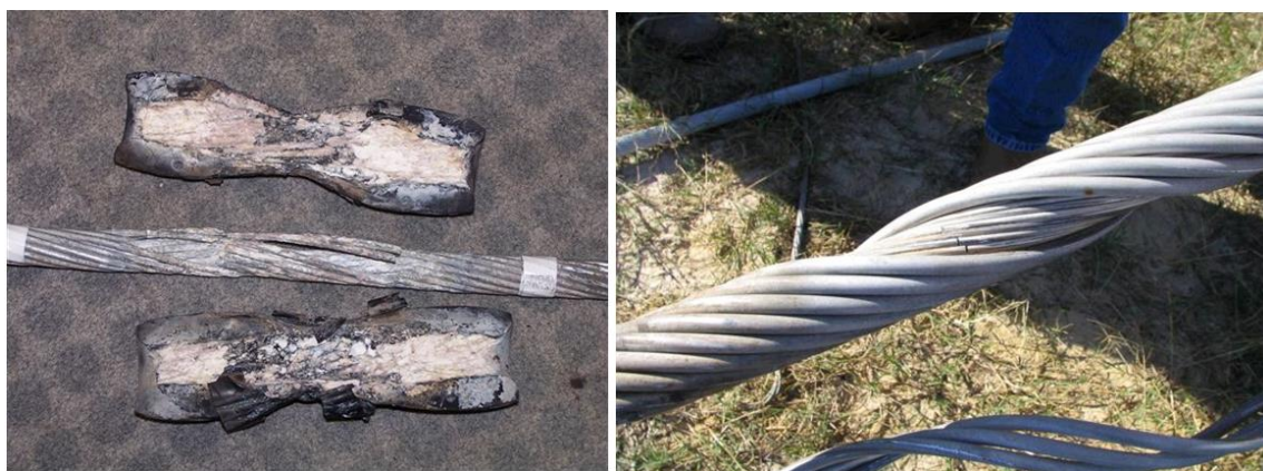
Damage Strands found inside suspension unit and under rods
