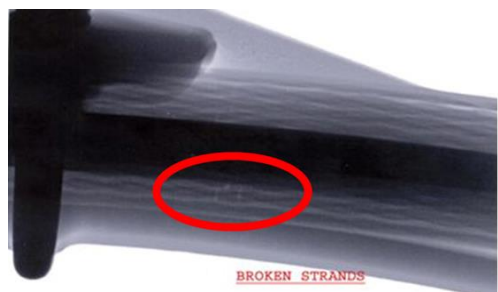
X-Ray of Broken Strand in a Suspension Clamp
