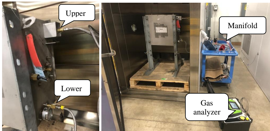
Figure 5: Low temperature test arrangement
