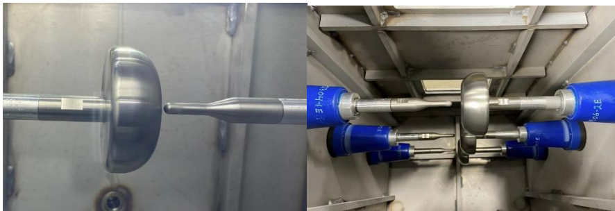
Figure 2: Round to plane electrodes (left) and arrangement of electrodes in tank (right)
