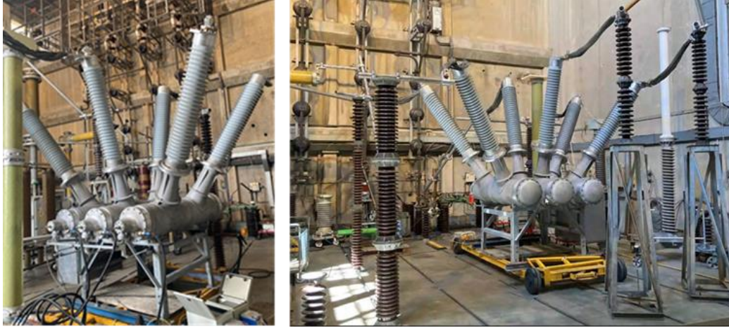
Figure 3. DT1-145g during power breaking tests at CERDA.
