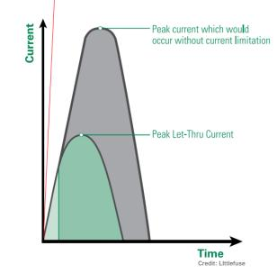
This race against fuse clearing time and DC rise is where we can discuss the possibility of a current limiting fuse
