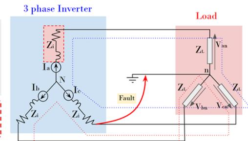
Figure: 3 phase inverter under SLG
