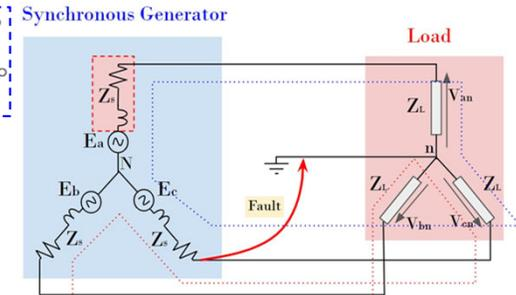
Figure: Synchronous Machine under SLG
