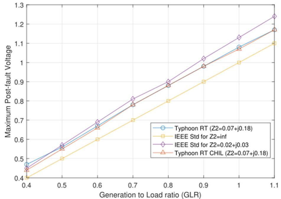
Figure: GFOV vs GLR (Experimental observation and IEEE Std)
