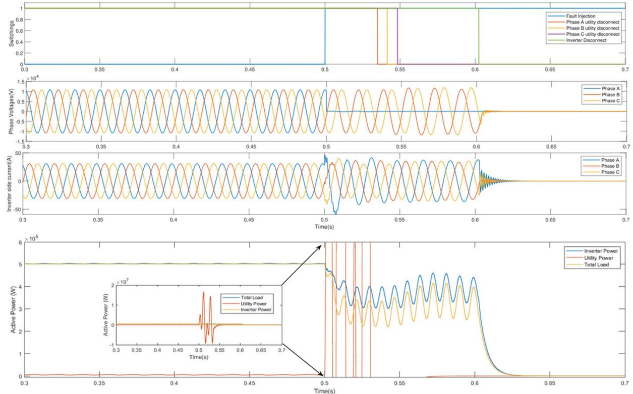
Figure: (a) Switchings (b) Phase Overvoltages (c) Inverter Currents (d) Active power fed into the system - in the GFOV experiment
