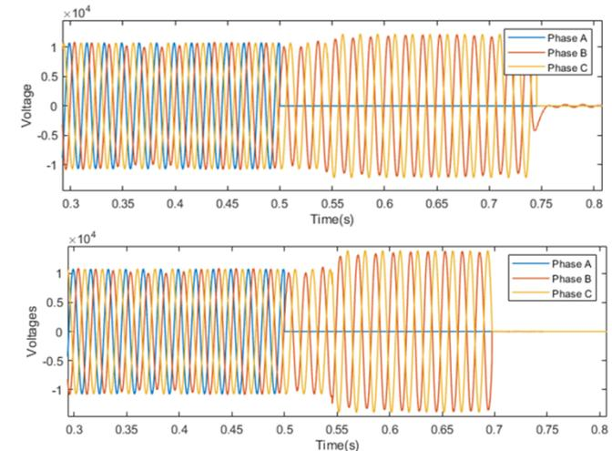
Figure: (a) Overvoltage with GLR=1.0 and pf=0.9
