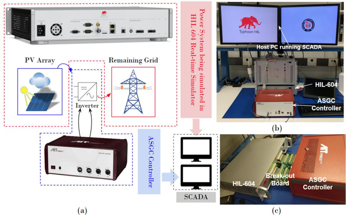
Figure: (a) Pictorial representation of the experimental setup, (b) The physical experimental setup, (c) The interface between ASGC controller and Typhoon HIL 604
