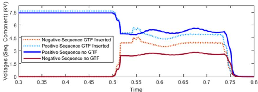
Figure: The sequence components of the voltages with and without the GTF in the system
