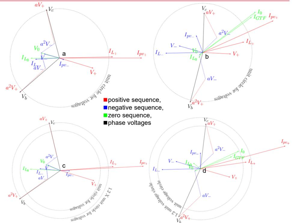
Figure: Phasor Diagrams for (a) GLR=1, no GTF | (b) GLR=1, with GTF | (c) GLR=1.2, no GTF | (d) GLR=1.2, with GTF
