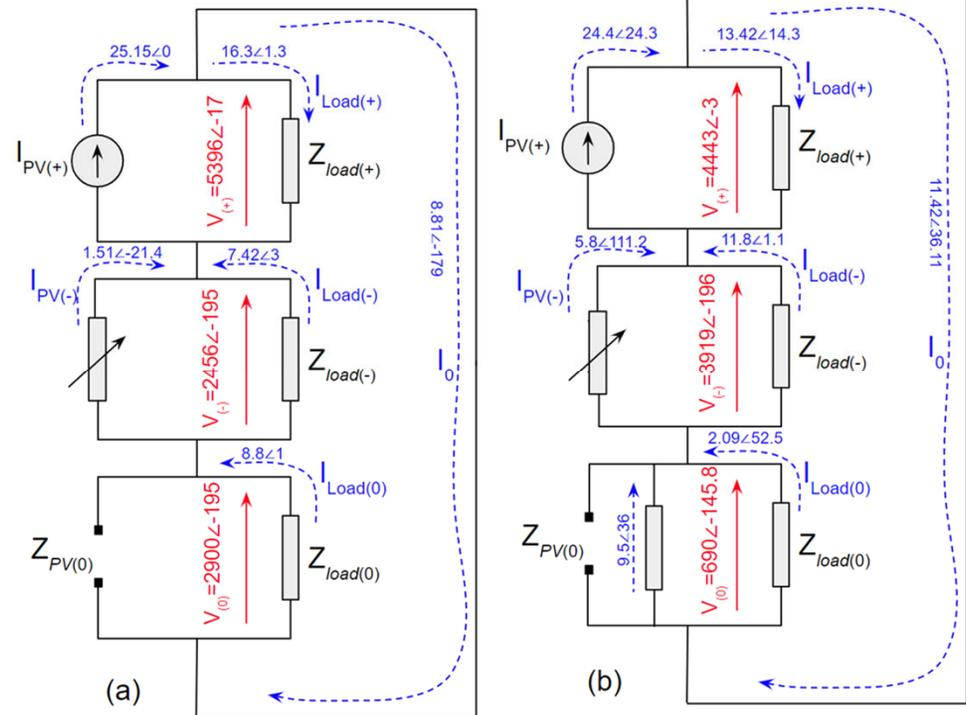
Figure: (a) A snapshot of the sequence diagram of the IBR under SLG without GTF at 0.625s
