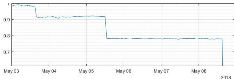
Figure 9 SCADA record of the voltage measurement before CCVT failure
