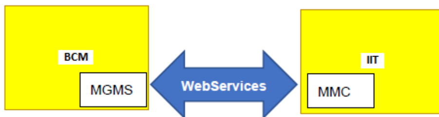
Figure 6. Microgrid clustering interface between the two microgrid controllers
