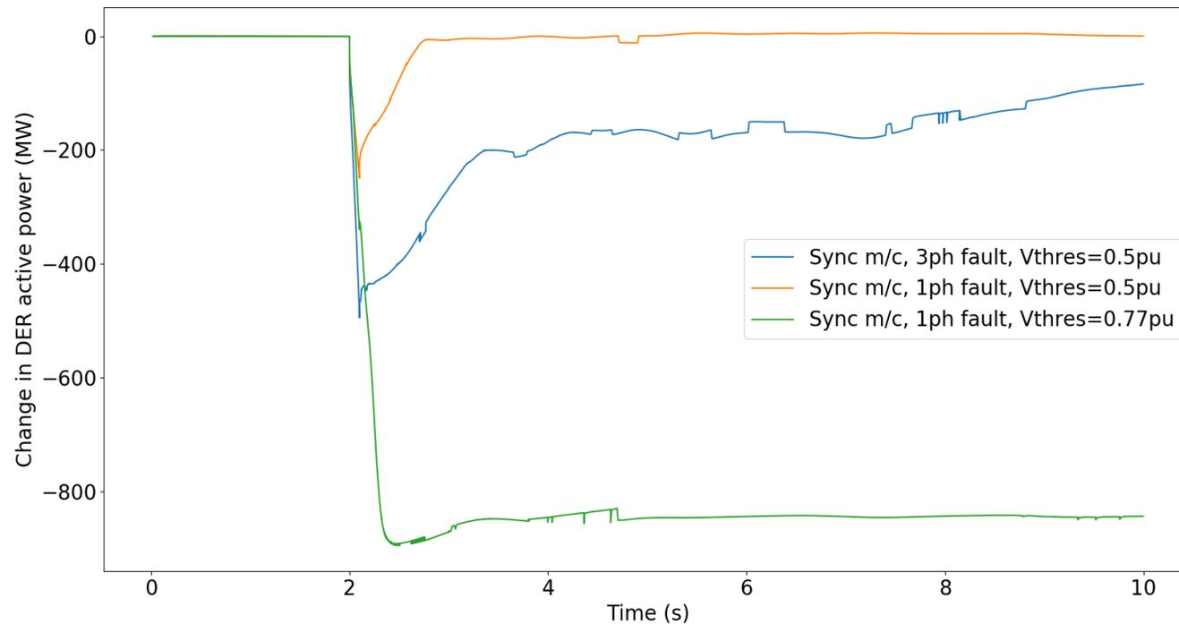
Without the parallel trip characteristic, there could be a huge misrepresentation of amount of DER that ride through a single phase fault
