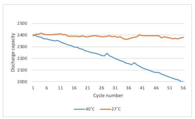
Measured decrease in discharge capacity (in mAh) of INR-25R cells at 40°C and 27°C over 55 cycles.
