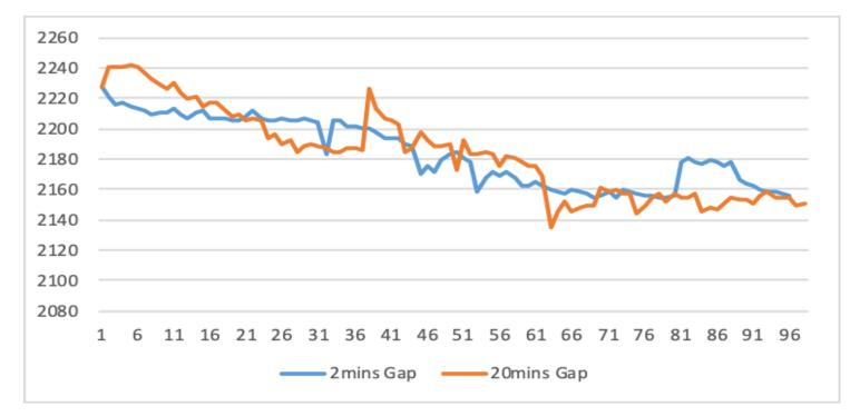
Measured decrease in discharge capacity (in mAh) of two INR-25R cells at 27°C over 100 cycles. Charge/discharge delay times were 2 minutes (blue curve) and 20 minutes (orange curve).
