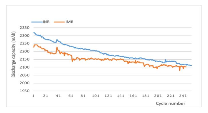
Measured decrease in discharge capacity of INR-25R and IMR-25 batteries over 250 cycles at 27°C.
