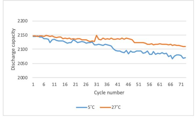
Measured decrease in discharge capacity (in mAh) of INR-25R cells at 27°C and 5°C over 70 cycles.
