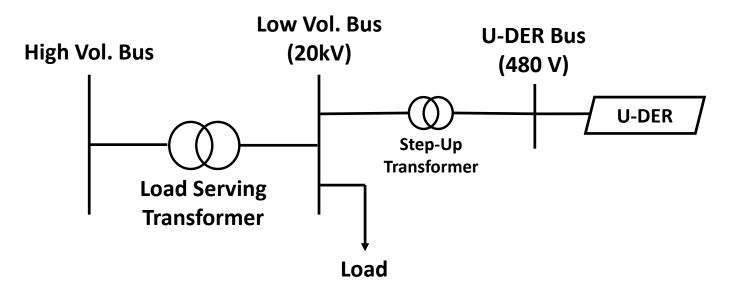
> Each U-DER is rated at 5 MVA, & is connected close to the load serving transformer
