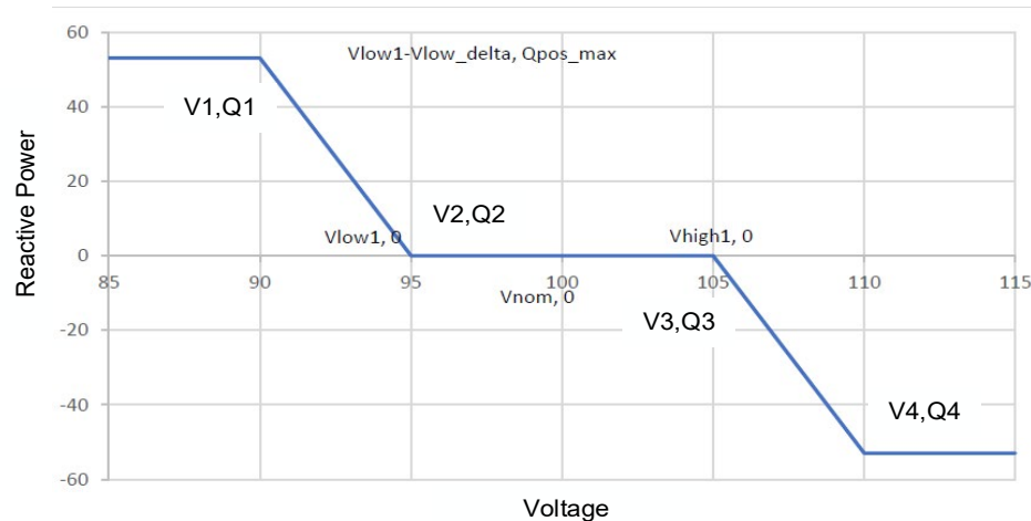
Example of setting for Volt-var mode
