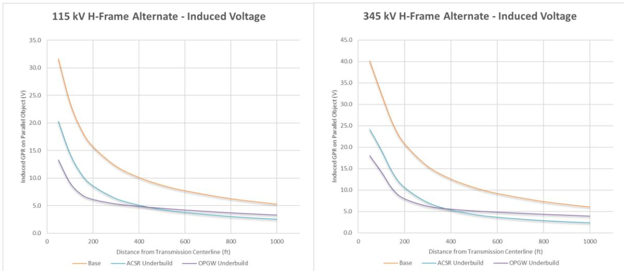
Figure 5: H-Frame Results Alternate OPGW Location
