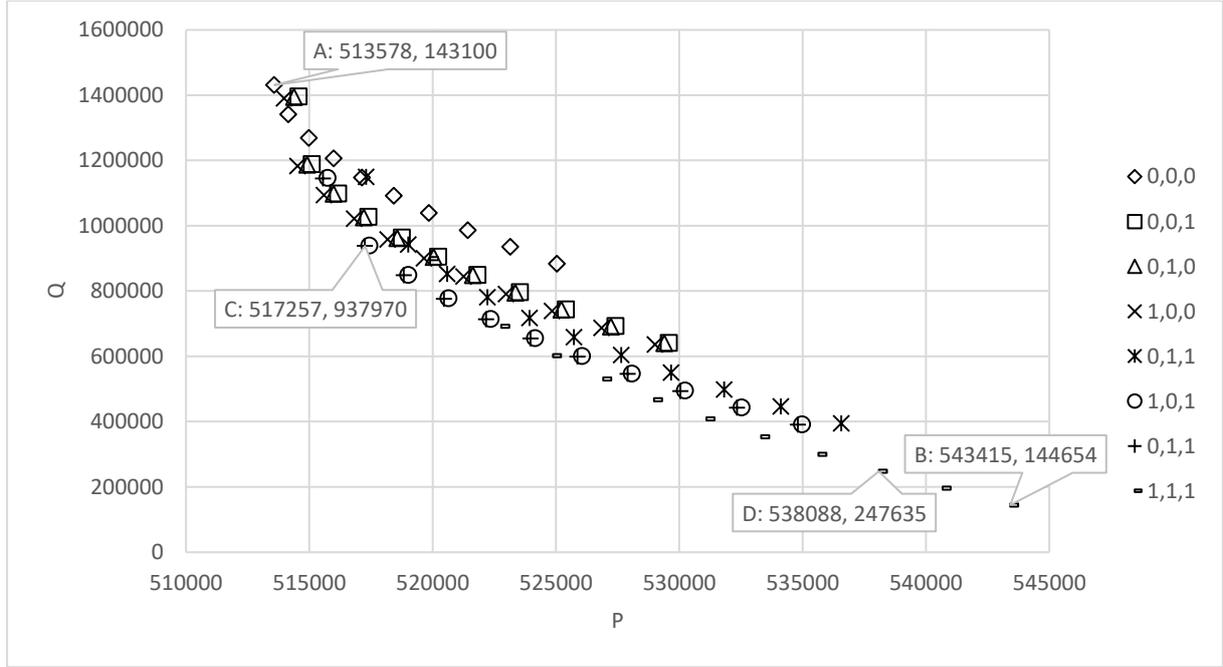
Figure 2: Calculated active power ( $P$ ) and reactive power ( $Q$ ) for all control points in the test feeder, with highlighted points of interest
