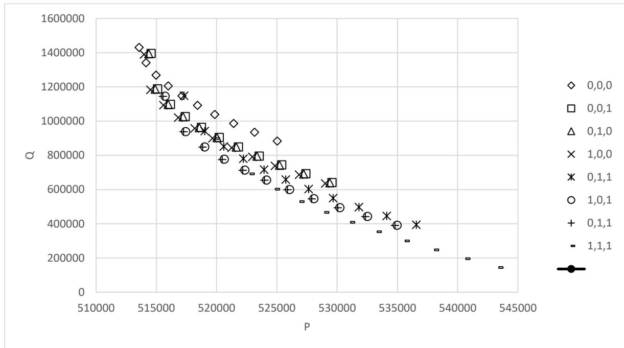
Figure 3: Active power ( $P$ ) and reactive power ( $Q$ ) on test feeder with efficient curve highlighted and  $\alpha$  values
