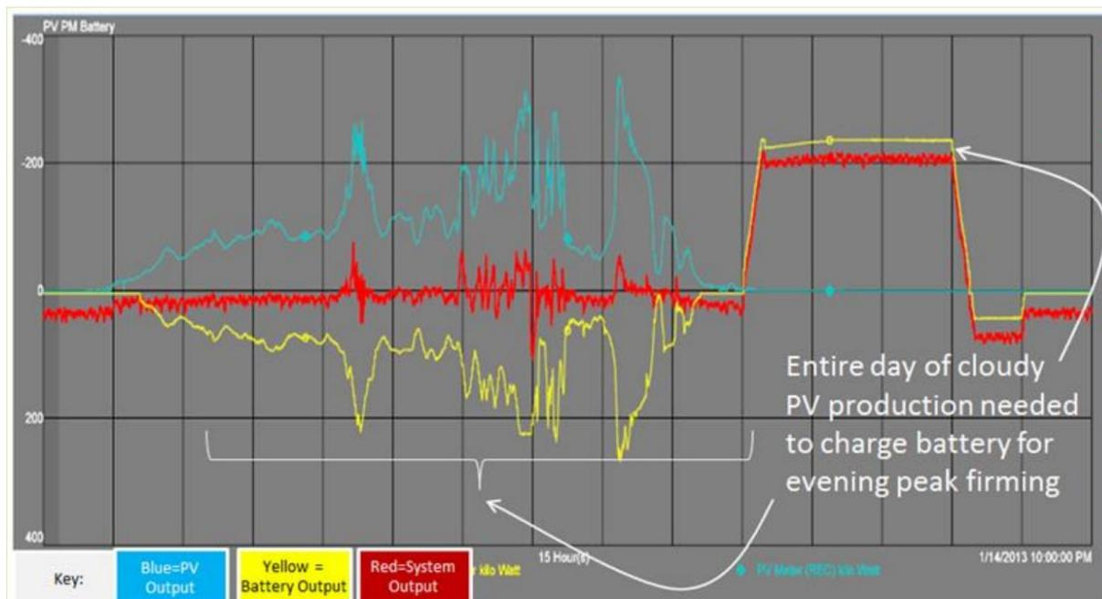
**Figure 5. Example of an ESS Performing Generation Firming of an Intermittent Resource Combined with Load Firming of the Evening Demand Peak [6].**
