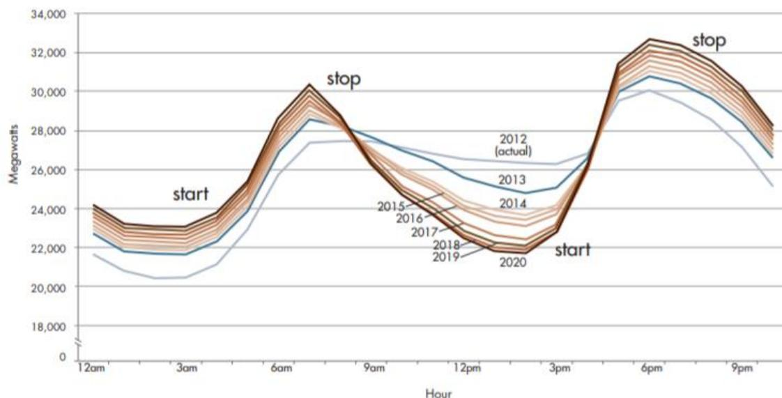
**Figure 4. Net Load on January 11 (Source: California Independent System Operator)**
