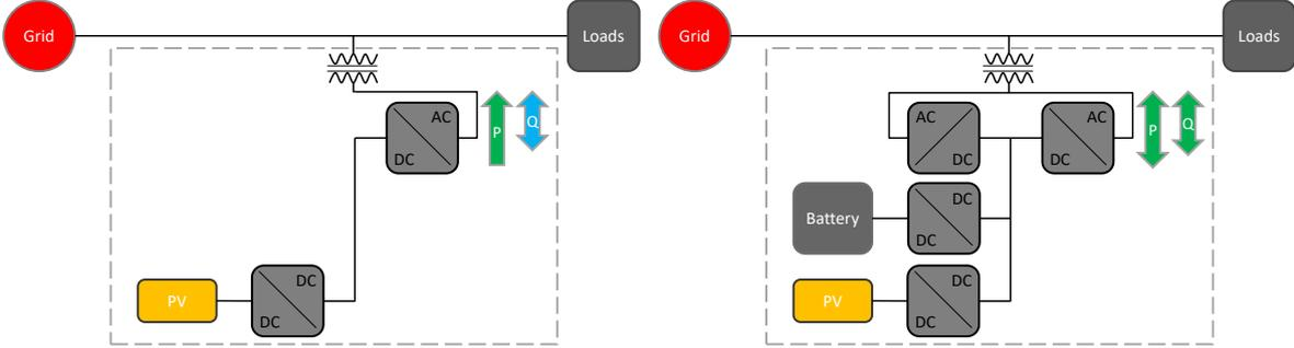
**Figure 2. Schematic of a Two Quadrant Inverter (Left) versus a Four Quadrant Inverter (Right)**
