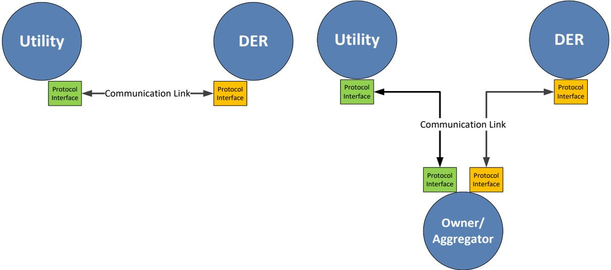
**Figure 3. Simplified Topology for Communication between Utility and DERs using Smart Inverters**
