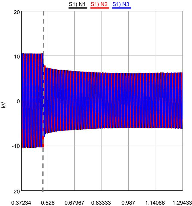
**Fig. 7: 13.2kV t=0.5 sec fault**
