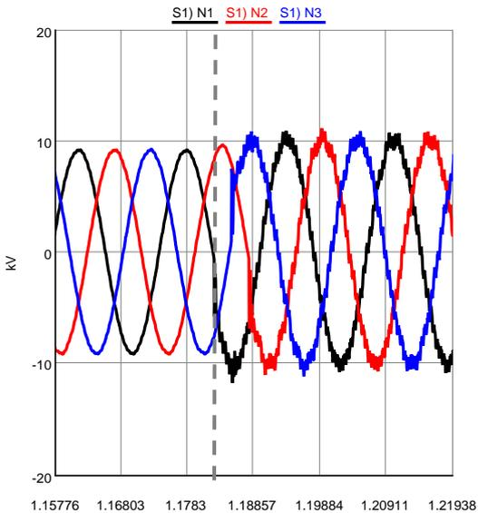
**Fig. 6: 13.2 kV t=1.18 sec 51 operation**
