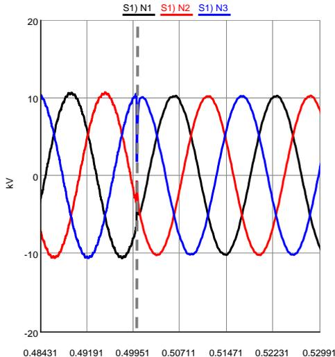
**Fig. 3 – 13.2 kV t=0.5 sec fault**
