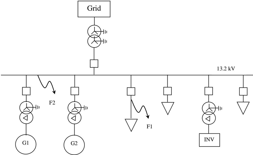
**Fig. 2: Microgrid Case Study 1-line Diagram**
