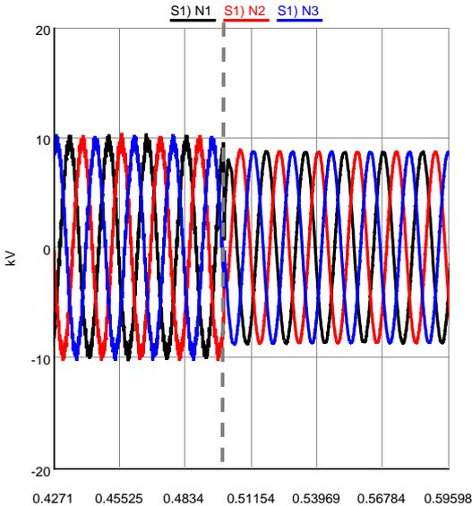
**Fig. 5 – 13.2 kV t=0.5 sec fault**
