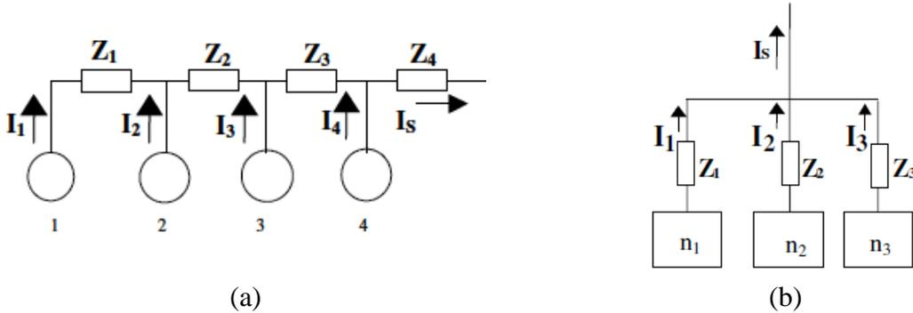
Figure 2 a) Sample Series Feeder; b) Sample Feeders in Parallel [1]
