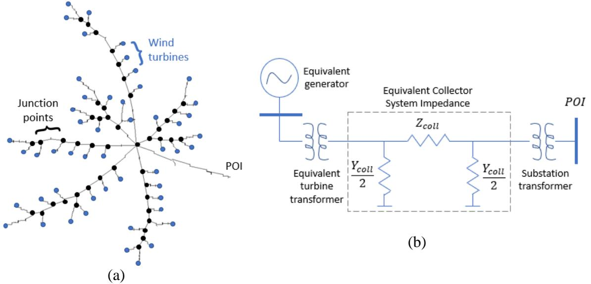
Figure 1 a) Full Wind Farm Connection Diagram; b) Aggregate Wind Farm Model
