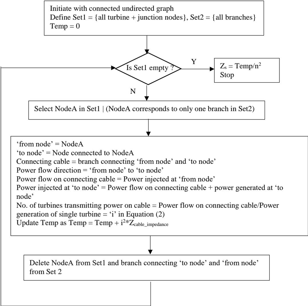
Figure 3) Algorithm for computing power flow direction and magnitude on different cable branches, along with  $Z_s$  per Equation (2).
