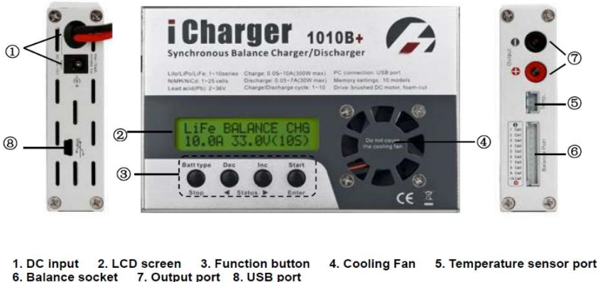
Figure 1. iCharger 1010B+ external controls and connections.
