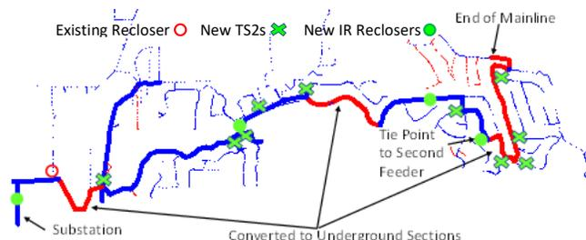
**Figure 5.** One-line diagram showing previous improvements, the addition of a tie-point low-energy fault-testing fault interrupter (IR) and existing device locations.
