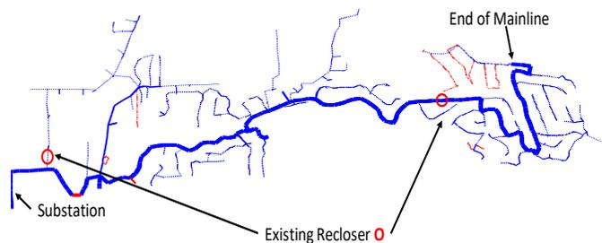
**Figure 1.** One-line diagram of example distribution feeder used for analysis.
