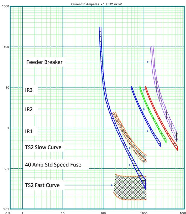
**Figure 7.** TCC curves selected for example feeder devices. Note: TCC curves are truncated at the maximum available fault current for their respective devices
