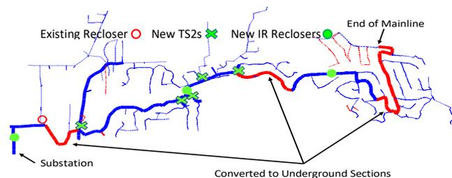
**Figure 3.** One-line diagram with two additional low-energy fault-testing fault interrupters (IR), 5 additional cutout-mounted recloser (TS2) devices, underground conversions and existing device locations shown.
