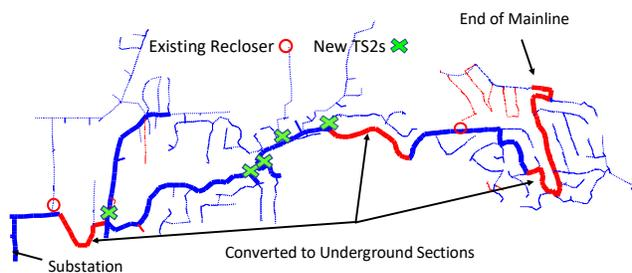
**Figure 2.** One-line diagram with the addition of 5 cutout-mounted reclosers (TS2), sections changed to underground construction and existing devices.
