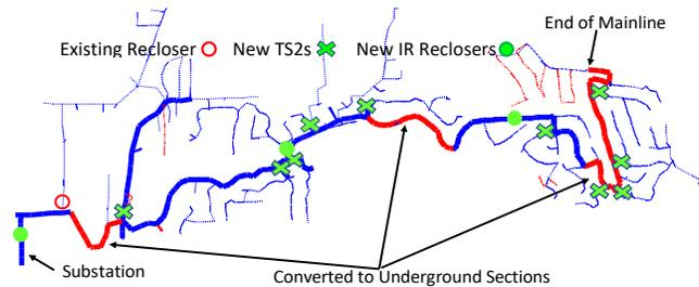
**Figure 4.** One-line diagram with 5 additional cutout-mounted recloser (TS2) devices, previous improvements and existing device locations shown.
