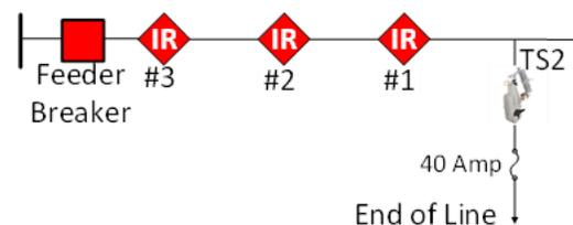
**Figure 6.** One-line diagram with coordinated series low-energy fault-testing fault interrupters.
