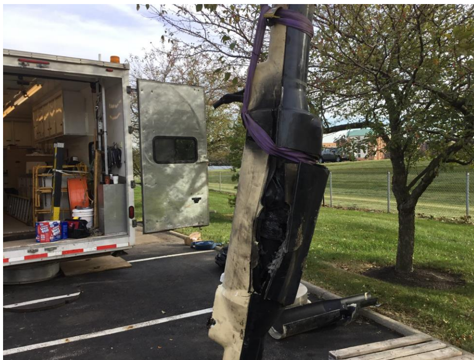
Figure 10: Manhole 4 Phase A failed cable splice for Circuit #1
