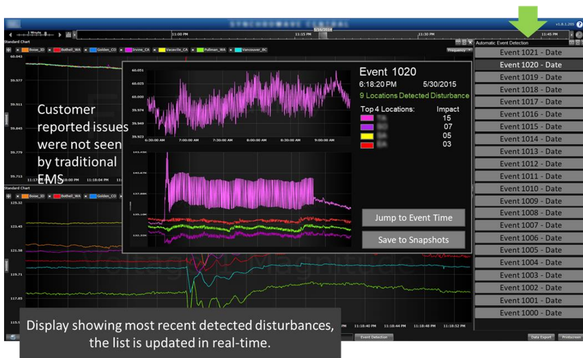
Figure 7 – STATCOM Oscillation Captured by Engineering PMU Data Client System
