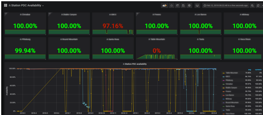
Figure 3 – Display of PMU data stream availability monitoring
