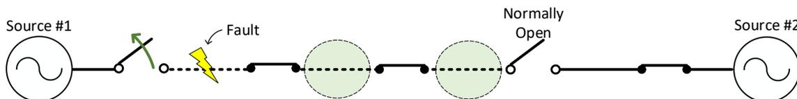
Figure 1: A fault appears on a radial network and is cleared by an upstream device. Three sections are unpowered as a result; one contains a fault, and the two circled sections are healthy and ready to be restored by the alternate source.
