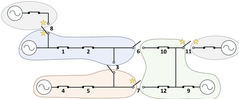
Figure 5: Network in steady state, with 5 feeders covering the area encircled. Stars are shown above open tie devices, on the side of which they are leaders of the feeder.
