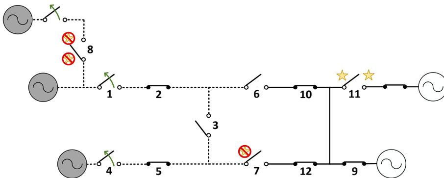
Figure 6: In this scenario the three sources on the left, colored grey, are lost simultaneously. Here the switches connected to the sources (devices #1 & #4) are set to open upon a loss of the source. Additionally, the leaders in each of the de-energized feeders sensed a loss of voltage in the system, and no longer consider their feeder available for restoring neighboring feeders. This is represented by the removal of the star icon.
