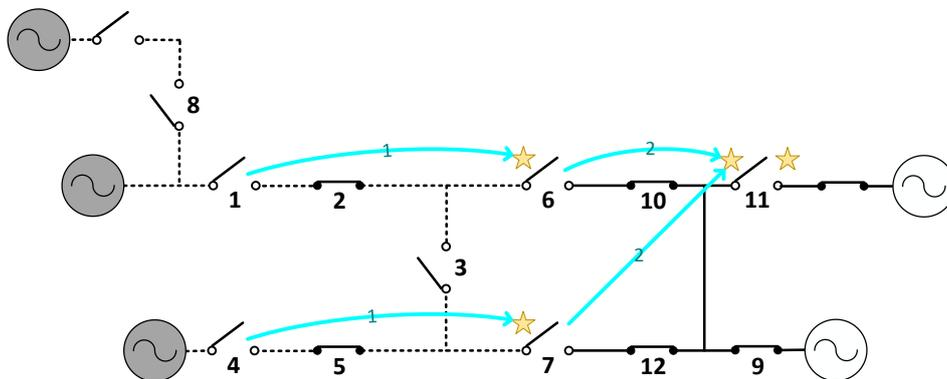
Figure 7: Devices #1 & #4 now inform the ties in their de-energized feeder that the source is isolated, and restoration can begin. Device #6 & #7 independently decide to close themselves to power their respective feeders. They both ask for permission from the leader of the powered feeder to close.
