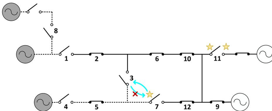
Figure 9: Device #7 knows that device #3 is a tie and attempts to get permission to close it as an alternate solution. The permission is denied by the tie, as it sensed a recent voltage loss in its feeder. Device #7 can periodically attempt to get permission for itself or device #3 to close. Once steady state has been arrived at again, and enough capacity is available, one of the devices can close.
