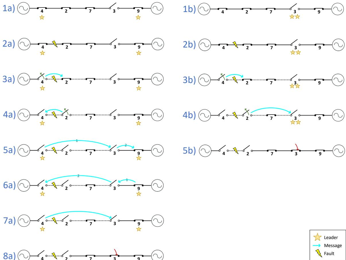
Figure 4: Diagram showing results from arbitrary leader vs tie-based leader. In scenario ‘a’ on the left, the restoration took place using 7 messages in 8 steps. In scenario ‘b’, where the leader was in the tie device, the restoration used 2 messages in 5 steps.
