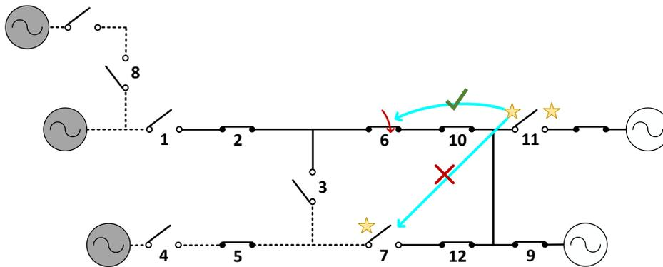
Figure 8: The leader of the powered feeder only approves one of the ties to close. It is a race condition in this example for which tie will be allowed to close, as the source may be overloaded if both are allowed to close. Here, device #6 is approved to close and does; powering the sections to its left. Device #7 is denied and remains open.
