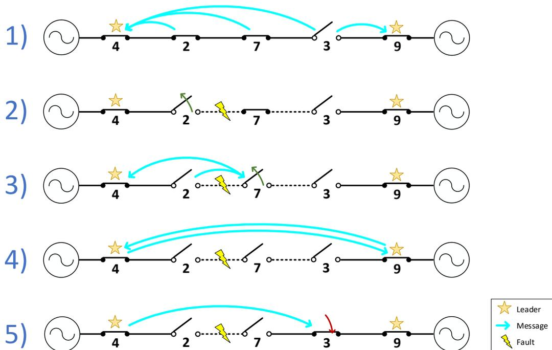
Figure 3: An example of the process of restoration under the distributed intelligence approach on a radial feeder connected to an adjacent feeder by a normally open tie point. Here a leader device is designated by the star and is device #4 in this example for the left feeder, and device #9 for the right.
