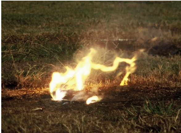
Figure 1 – Downed line arcing
