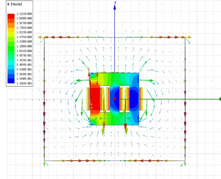
*Figure 5 Flux density distribution*
