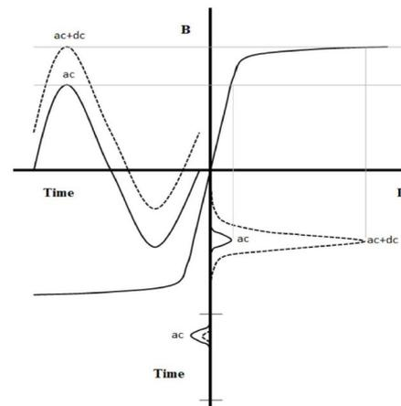
Provided the transformer undergoes partial saturation, the following effects are possible
