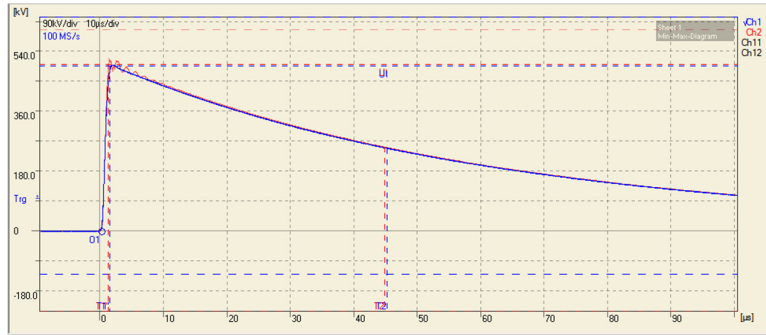
Figure 9: Lightning impulse behaviour – GIS type RGK 400DC [11]
