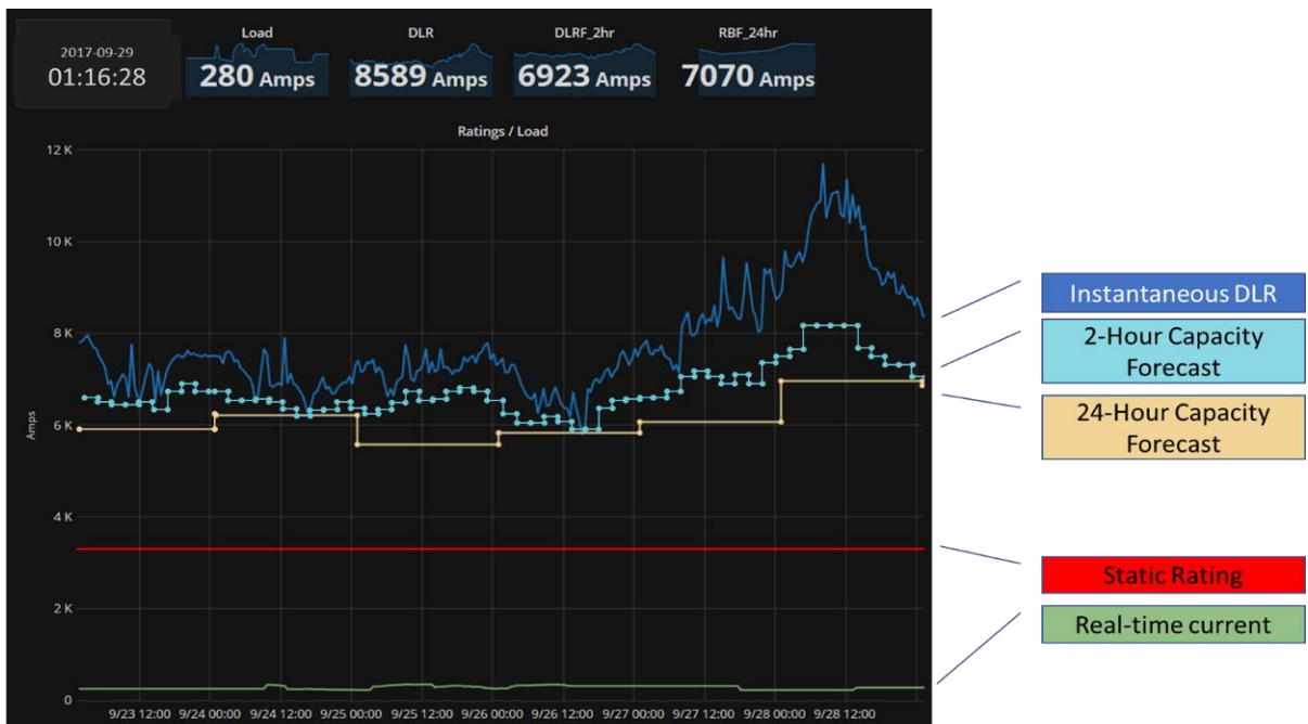
Figure 5: Forecast DLR Output showing 2- and 24-hour ahead forecasts on a 735kV line. Ratings in Amperes.
