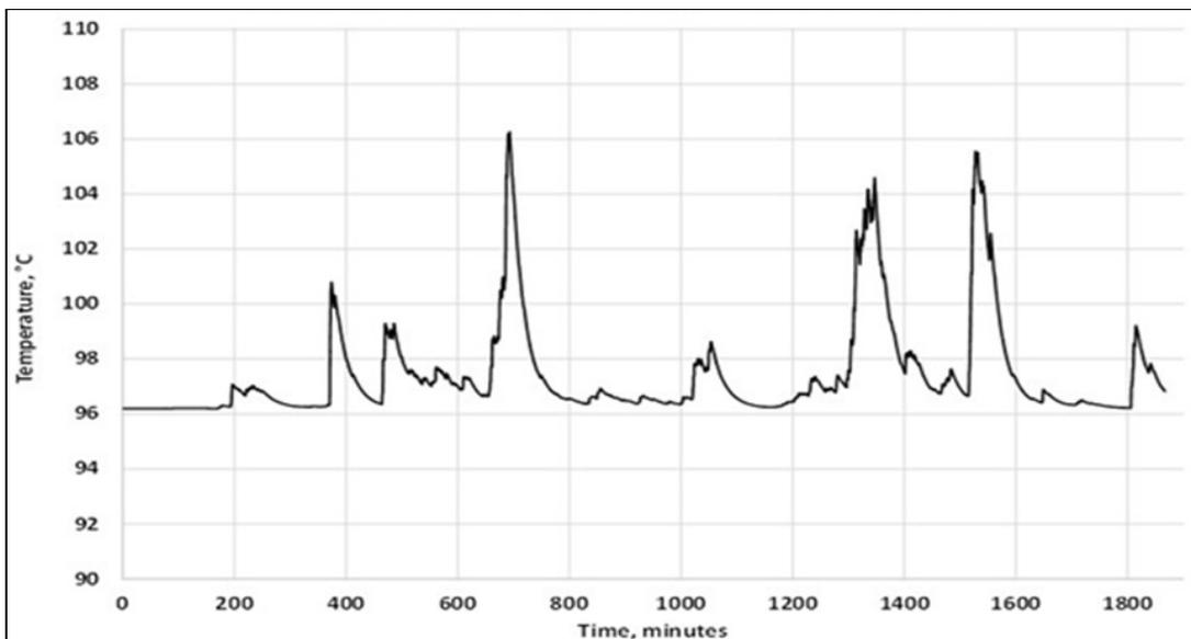
Figure 4: Calculated Tank wall hot spot temperatures of transformers at Weakley Substation corresponding to GIC Signature of Figure 1 (b)
