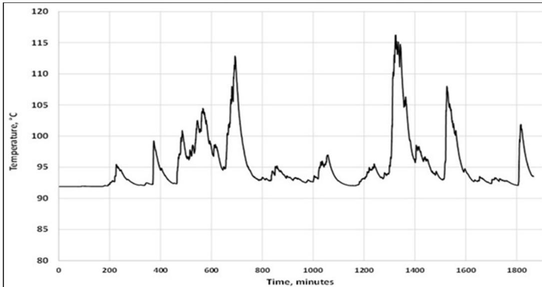
Figure 3: Calculated Fitch plate hot spot temperatures of transformers at “Paradise” Generating station corresponding to GIC Signature of Figure 1 (a)
