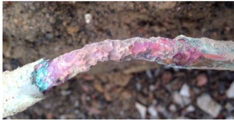
Fig. 11. Corroded ground conductor
