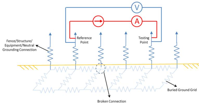
Fig. 12. Grounding integrity testing
