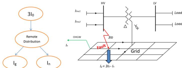
Fig. 4. SI method fault current distribution
