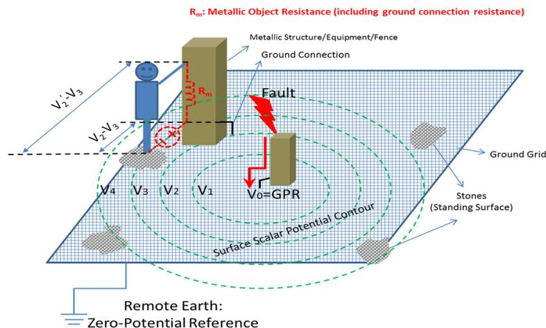
Fig. 1. Touch potential illustration when a ground fault energizes the ground grid
