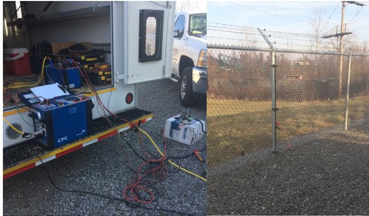
Fig. 13. Ground grid integrity testing set-up
