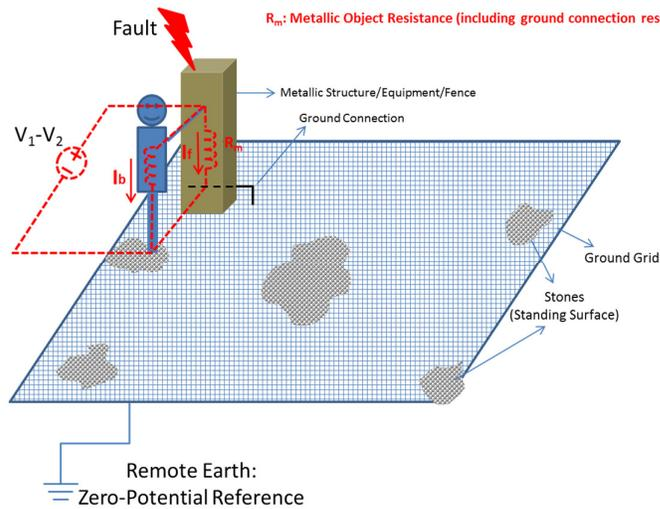
Fig. 2. Touch potential illustration when a ground fault energizes the fence/structure
