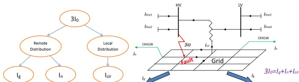
Fig. 5. MI method fault current distribution
