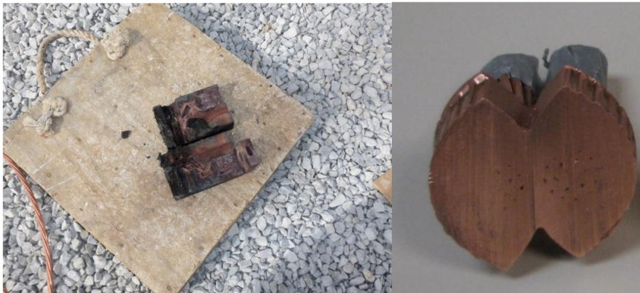
Fig. 10. Inconsistently welded connection (left) Swage connector cross-section (right)
