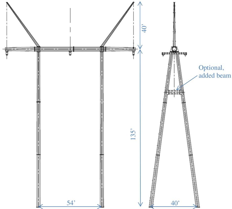
Fig. 3 Three phase dead-end structure with reported vibrations
