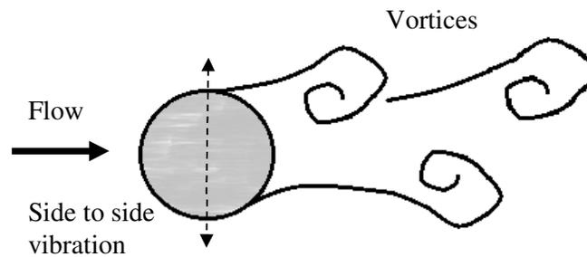
Fig. 1 Vortex shedding on a bluff body forming the vortex street
