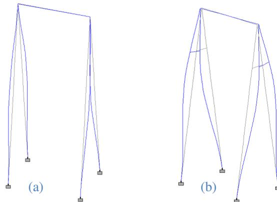
Fig. 4 (a) First observed mode of vibration, (b) second observed mode of vibration after addition of the short beams
