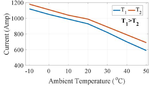
Fig. 2. Variation of ampacity as a function of ambient temperature
