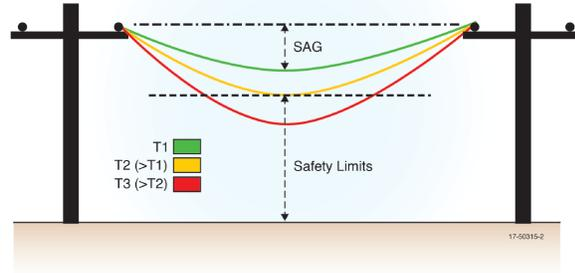
Fig. 3. Variation of sag as a function of temperature [16]
