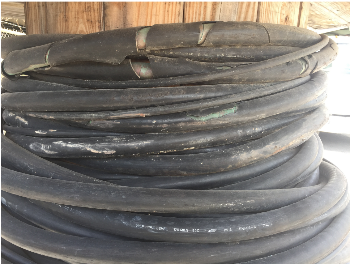
Figure 1: Cable Damaged by Elevated Temperatures Caused by Steam. Cable had been in Service for Only 2 Years.
