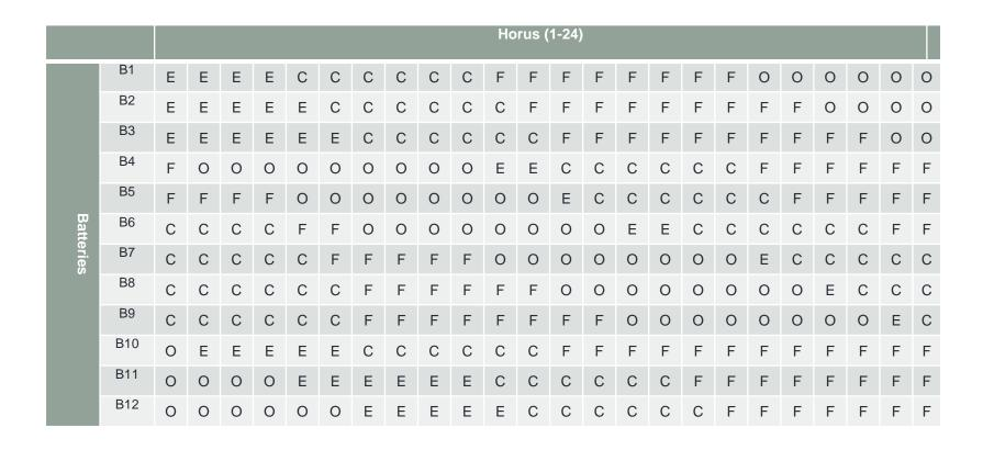
Each battery can have one of these four states at every hour: empty (E), charging (C), fully-charged (F), and out-of-station (O).
