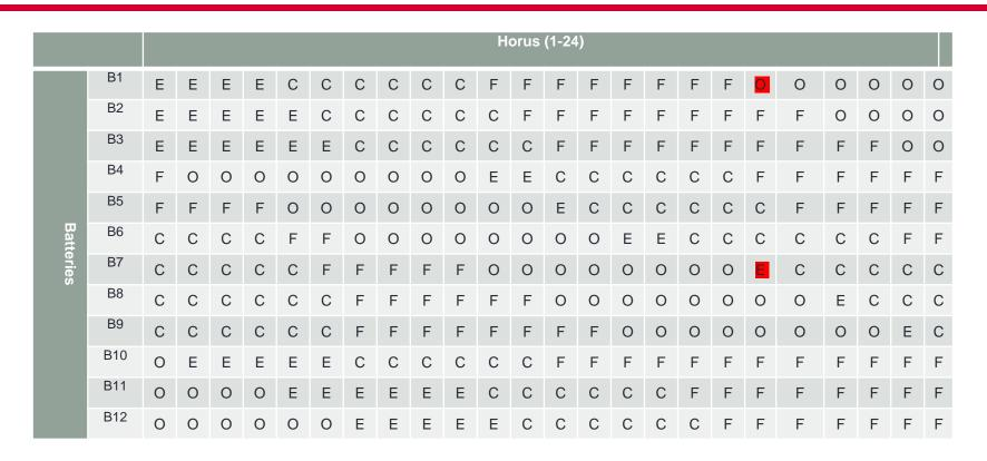
Battery B1 remains empty for the first four hours, and once one of the battery chargers becomes available, it starts charging. For the next six hours, the battery is charging until being fullycharged. This battery stays at fully-charged state because of lack of demand. At hour 19, battery B1 is swapped with battery B7
