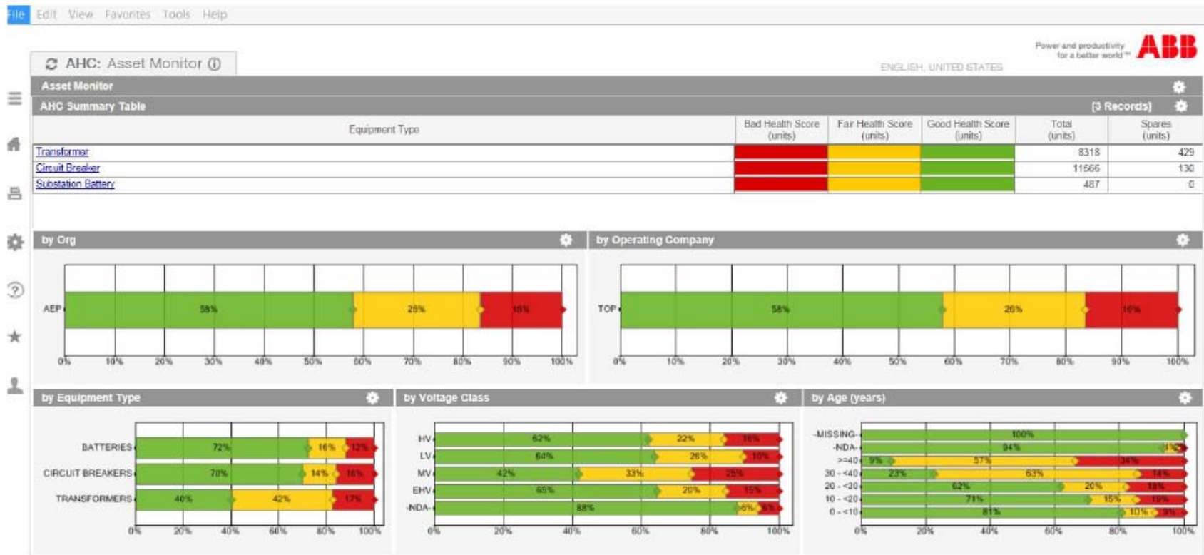
Figure 6 – The asset health solution top level screen of the solution showing classification of transformers and other assets in the red (requiring immediate attention), yellow (requiring some attention but not urgent) and in the green zones (may require attention but does not impact operational risk as is).
