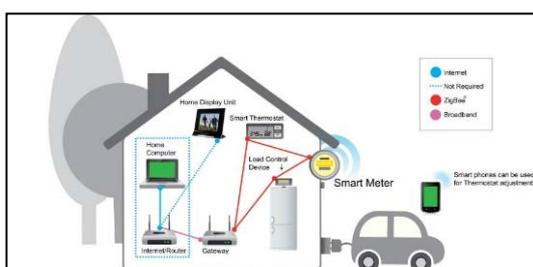
The meters selected and proposed for the Pilot will both measure the customer's energy consumption and report the consumption data in 15 minute increments to the Company. The meter will measure and report total consumption, interval consumption, demand, and energy supplied by the grid. The meters will be deployed to customers located within the Pilot area acting as a portal between in-home customer
