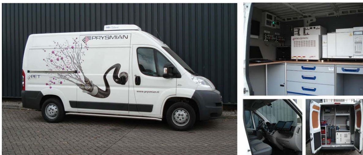
Photo 3 'PFT mobile laboratory for detecting small quantities of PFT in the atmosphere'
