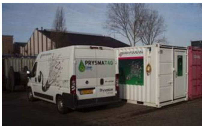
photo 2 'Equipment for injecting PFT in LPOF system during service'
