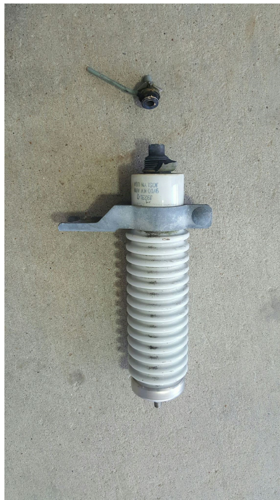
Figure 3: Failed lightning arrestor from Case Study 2
