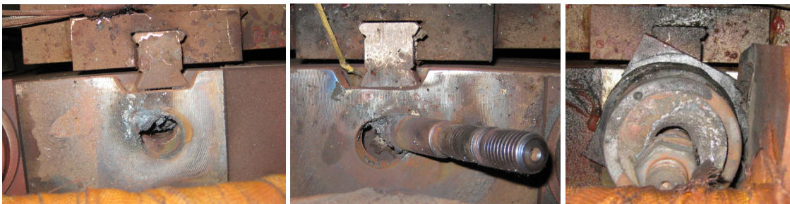
Fig 1. Melted through bolts and heated key bar
