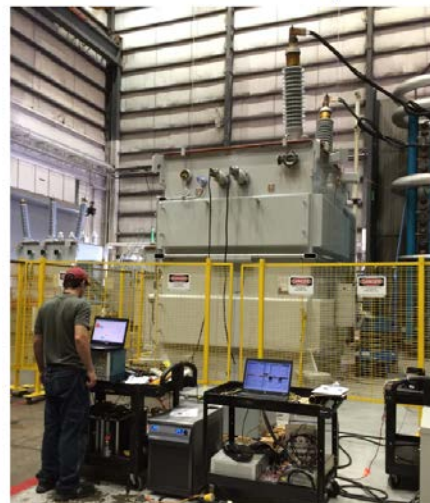
Magnetic Amplifier (MA) or Continuous Variable Series Reactor (CVSR)
