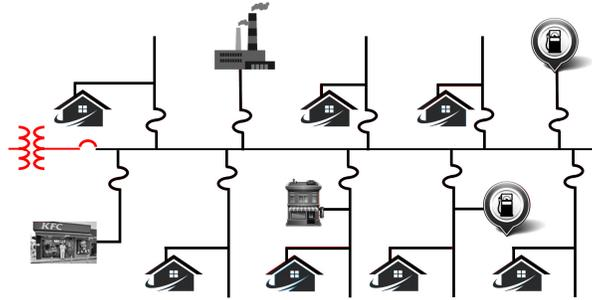
Figure 1: Substation breaker or recloser operates on a lateral transient fault. All customers down the breaker experience a momentary blackout.
