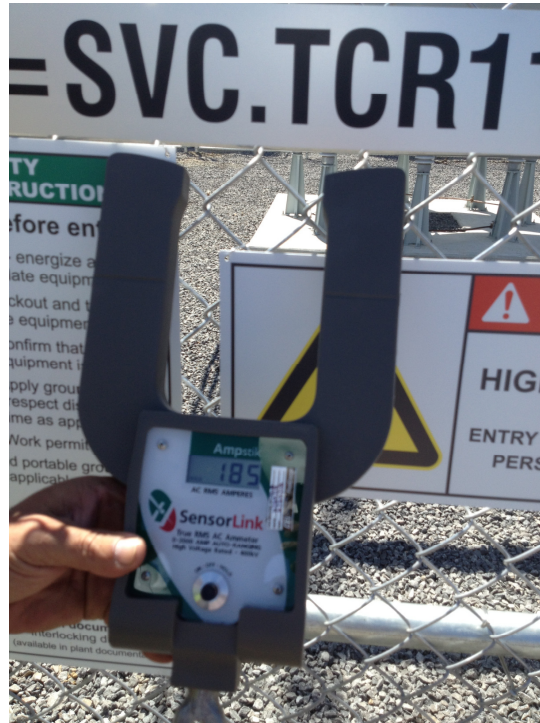
Figure 1: High Current in the TCR Branch Fence
